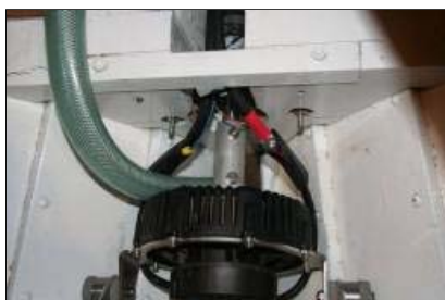
El-motor montert i Alphaboat
